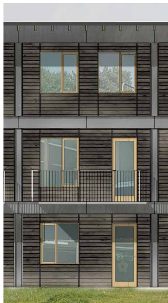
Facade study: Wood and steel sheets.
