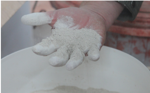
It was possible to remove the weakest of the three mortars in 10 seconds.
