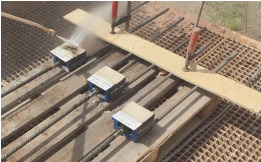
The lime mortar is flushed with a high pressure cleaner.
